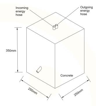
3) - The prepared anchor is embedded in the concrete and leveled.
